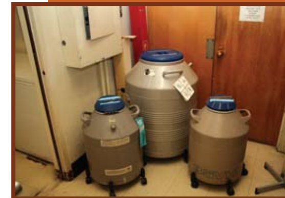
The cryogenic tanks contain liquid nitrogen, which stores critical samples at less than -320° F
