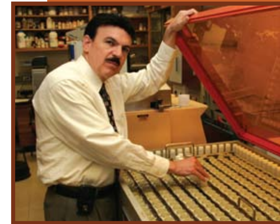
Dr. Rubin, using a scintillation counter, is determining the amount of radioactivity present in a sample
